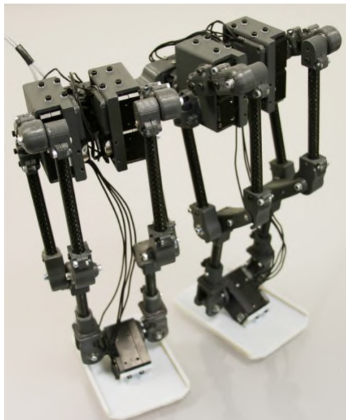
Figure 1.15: Example of a Serial-Parallel Hybrid Leg Mechanism [41]
