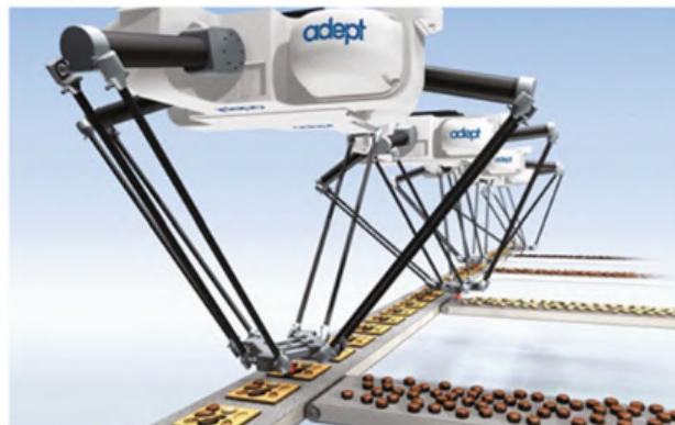
Figure 1.13: The pick and place Quattro parallel robot [39]
