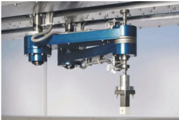
(a) The planar 5-bar mechanism [35]
