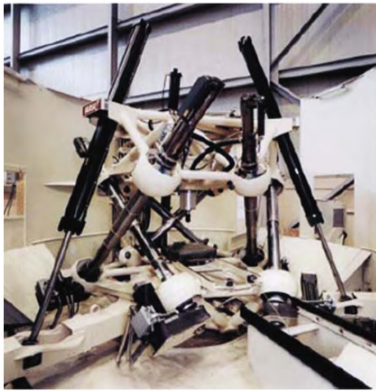
(a) The first milling machine based on the principle of Stewart platform [24]
