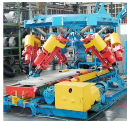
(b) The last Gough platform tire-testing machine
