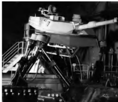
Figure 1.21: The turret motion-based simulator of the US army [9]
