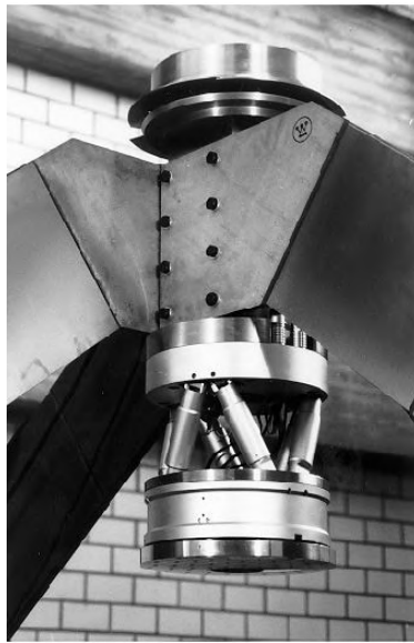
Figure 1.18: Hexapod used for secondary mirror alignment [9]
