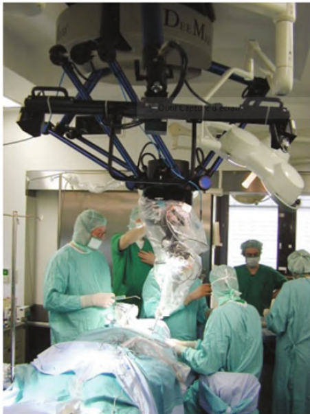
(a) Using Delta robot as a microscope stand by the ISIS system [40]
