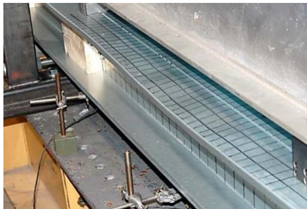
Figure 3.2: Local distortional buckling interaction in test beam [65].
