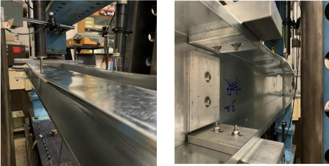
Figure 2.17: Evidence for L-D interactive mode from different perspective in Lipped-C beams [17].
