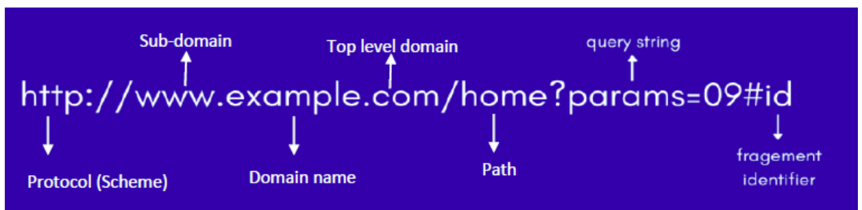
Figure 4.2: Parts of a URL structure [114].
