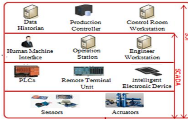
Figure 5.1 SCADA and ICS components
