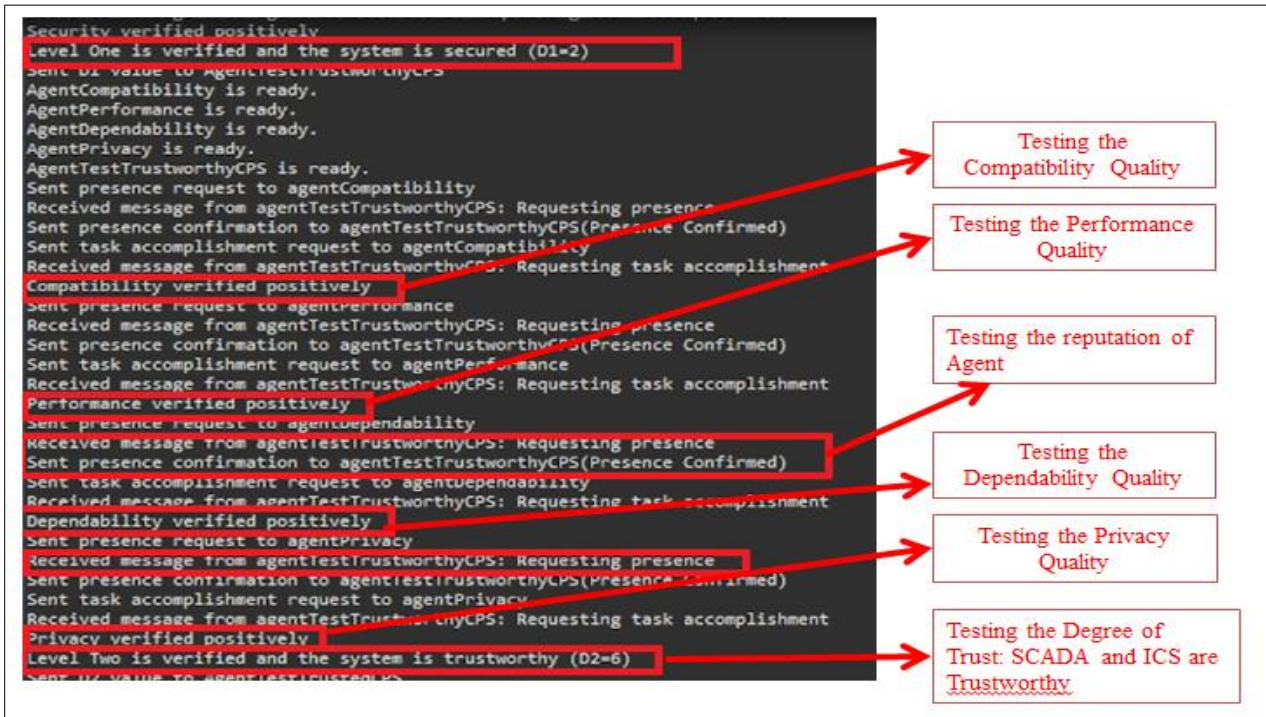
Figure 5.8: Test results for level two of trust petroleum SCADA and ICS systems
