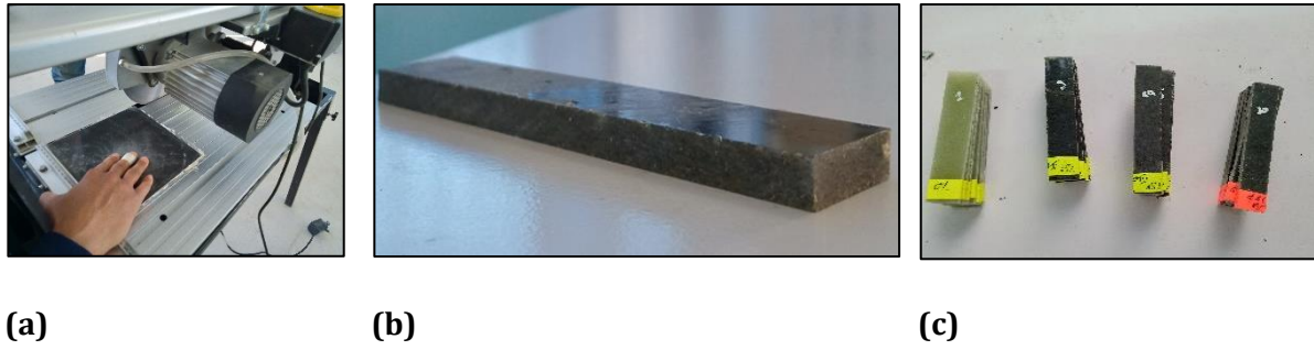
Figure II.6. Bending specimen's preparation.
