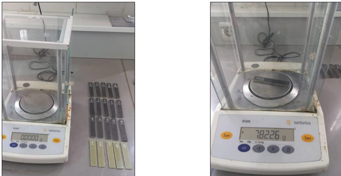
Figure II.10. Weight measurement operation
