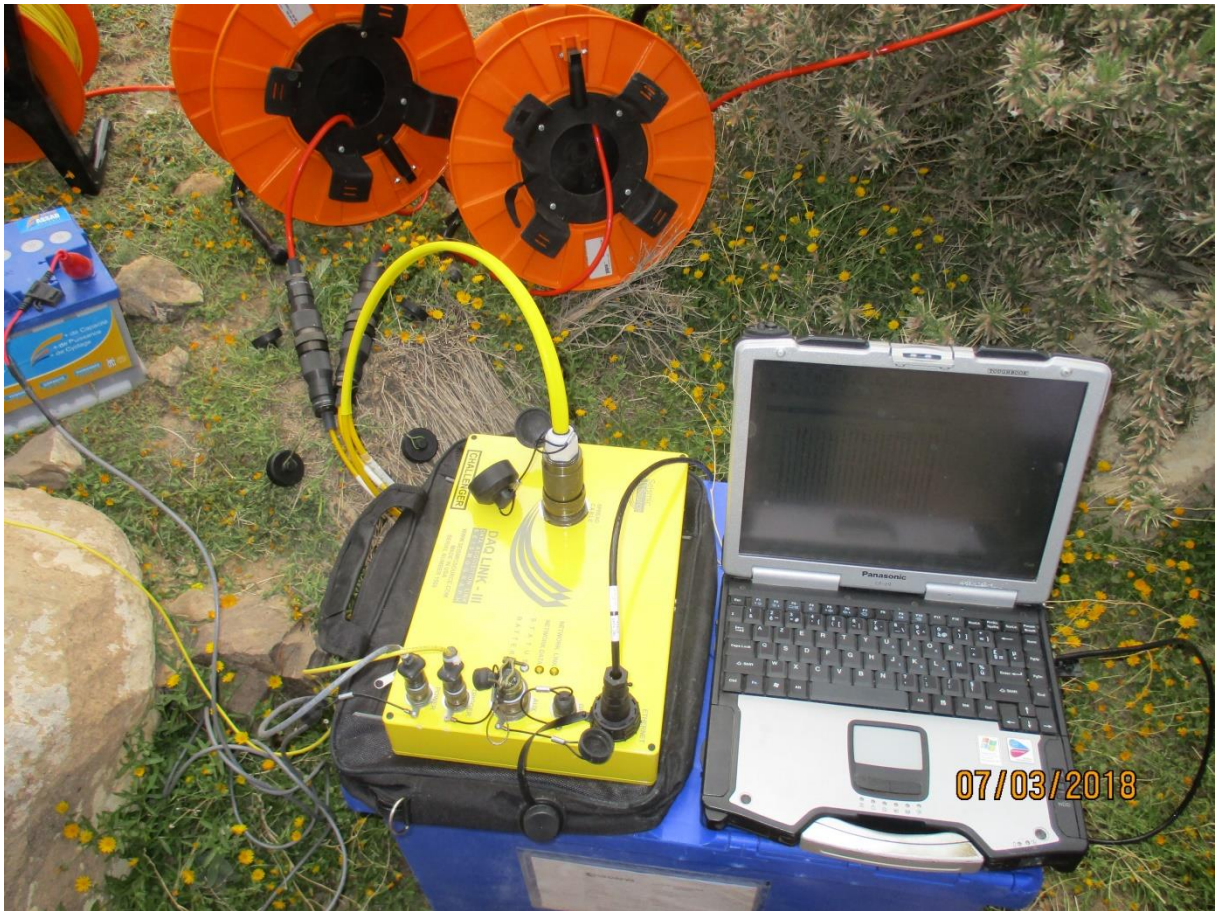
Fig .47: Sismographe DAQLINK III
