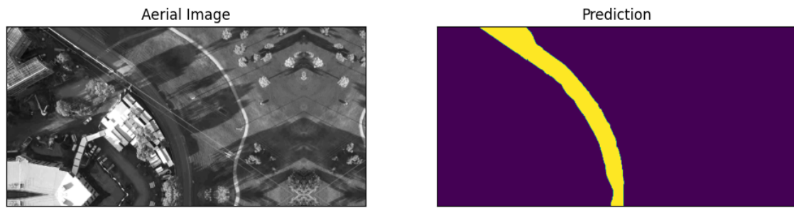
Figure 4.6: Semantic Segmentation of the Aerial Road Image with BGN-UNet
