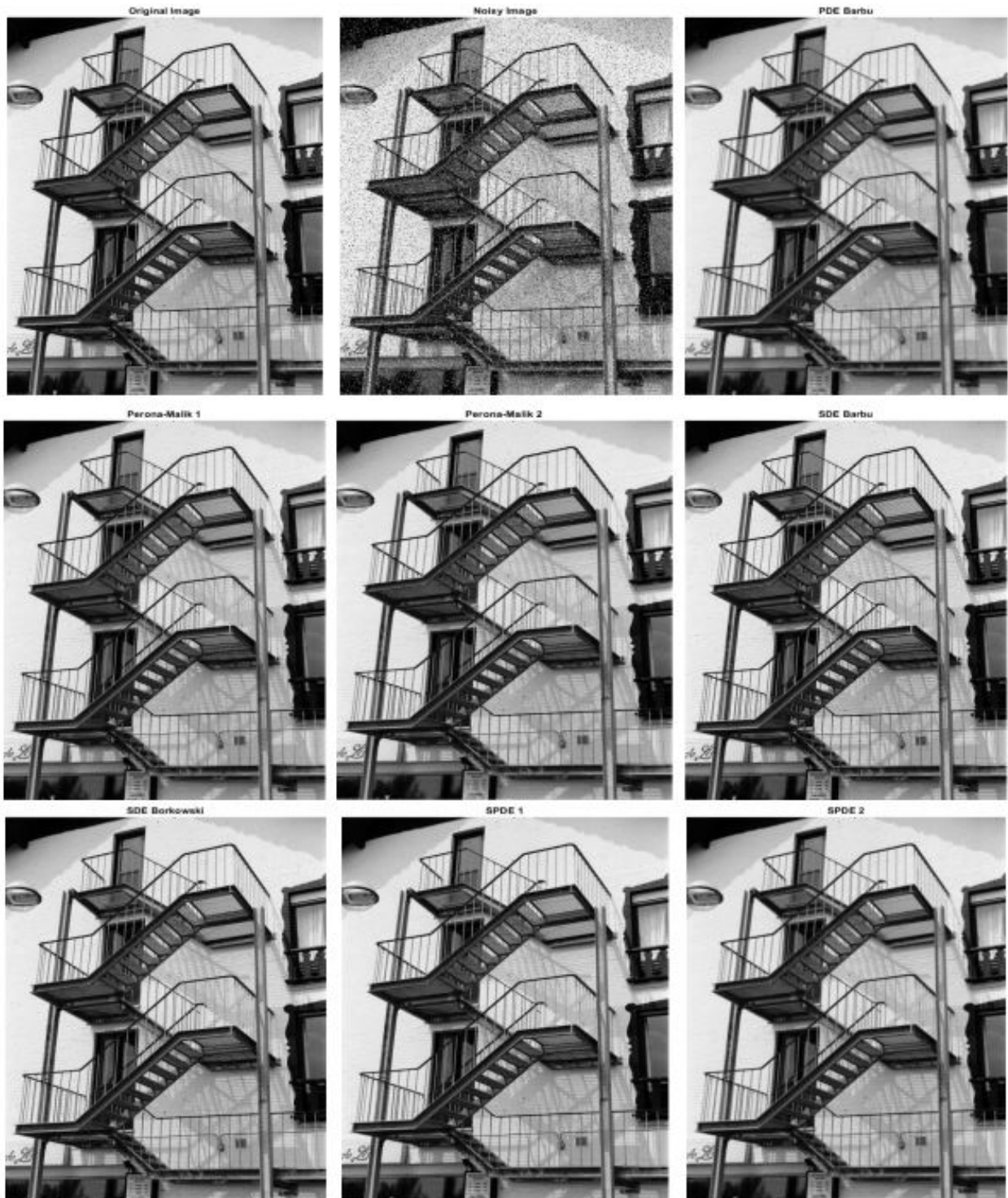
Figure 4.2: Restored image results after 'salt & Pepper' noise application with \Delta t = T/N , N = 5 , T = 1 , \gamma = 0.1 and \sigma = 0.45
