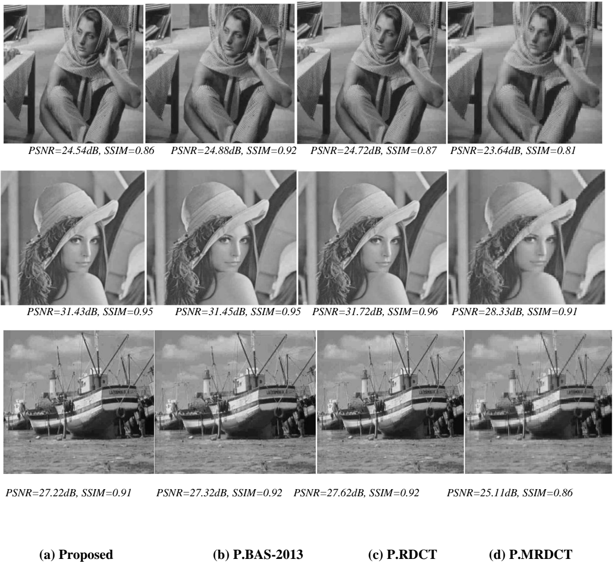
Figure.4.5. Reconstructed images at 0.35 bpp using different approximations.
