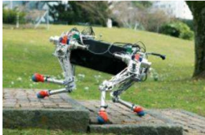
Figure 11: robot StarLETH quadrupel plateforme (Springy Tetrapod with Articulated Robotic Legs) image tirée de [43]
