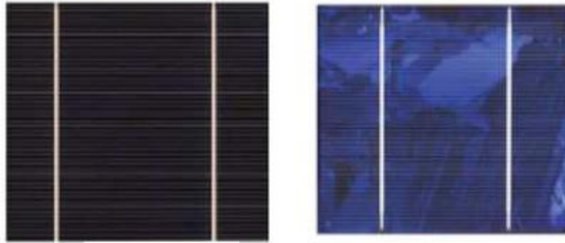
Figure 1.7. Cellules (a) monocristalline et (b) poly cristalline [46].
