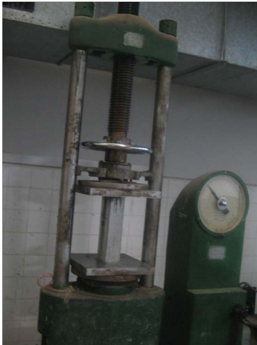
Fig3.4. Test arrangement for concrete filled tube testing.
