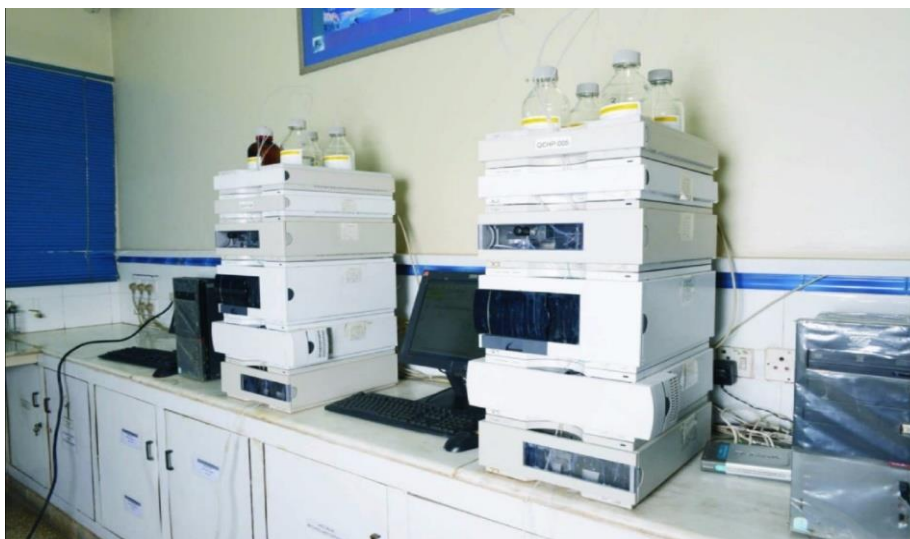
Figure 26 : appareil chromatographique (Agilent 1200 HPLC System)
