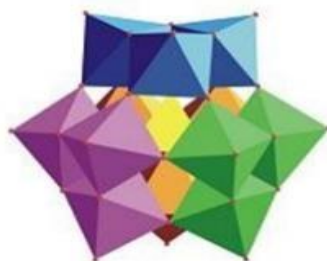
Figure I-12 : Description de la structure de Keggin.
