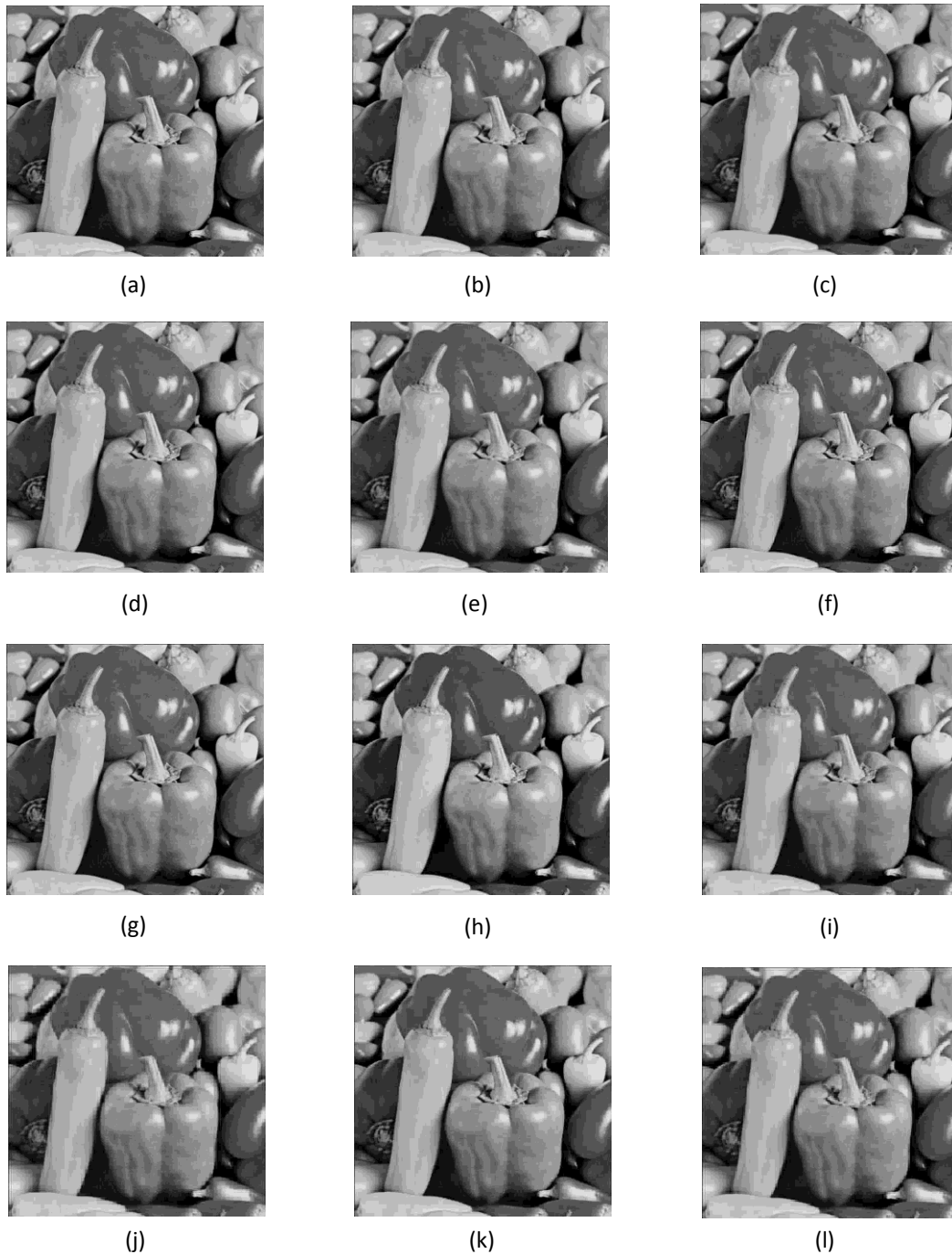
Figure 4.3. Image de test Peppers encodée à 0,5 bpp. (a) PSNR=33.96, SSIM=0.866 [Loeffler 1989]. (b) PSNR=31.81, SSIM=0.834 [Bouguezel 2013]. (c) PSNR=29.44, SSIM=0.839 [Kouadria 2013]. (d) PSNR=32.27, SSIM=0.841 [Cintra 2011b]. (e) PSNR=30.03, SSIM=0.831 [Mechouek 2016]. (f) PSNR=30.22, SSIM=0.811 [Tablada 2017]. (g) PSNR=33.54, SSIM=0.858 [Oliveira 2018]. (h) PSNR=30.89, SSIM=0.811 [Jridi 2017]. (i) PSNR=30.89, SSIM=0.807 [Bayer 2012]. (j) PSNR=26.97, SSIM=0.752 [Coutinho 2015]. (k) PSNR=30.61, SSIM=0.804 [Potluri 2014]. (l) PSNR=28.43, SSIM=0.780 [DCT proposée].
