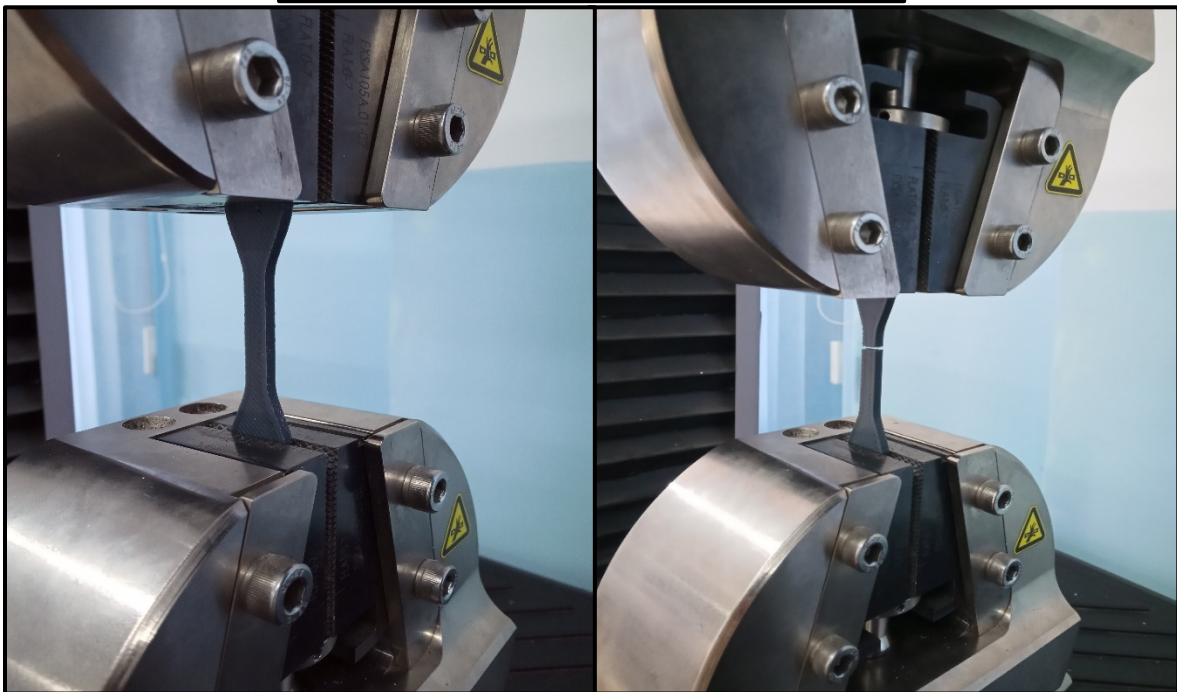
Figure 40 Top “the MTS Criterion Model43”, Bottom “tensile test before and after the specimen rupture”
