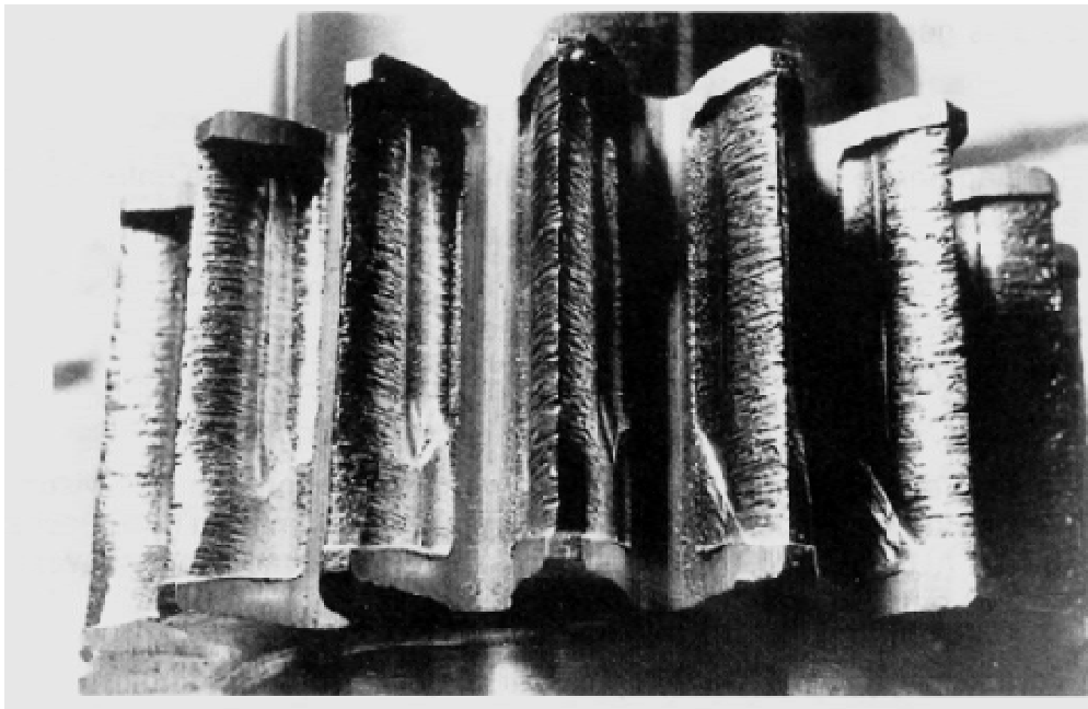
Fig. 46 Usure exagérée destructive [38]
