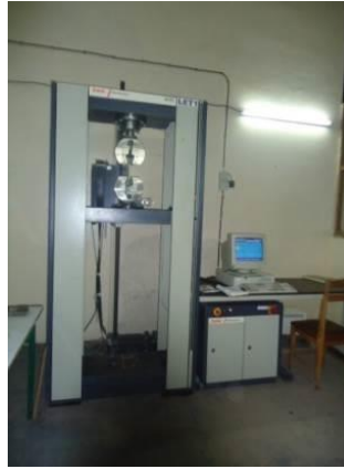
Figure IV.5 Machine de traction (ZWICK 1476 LET1)
