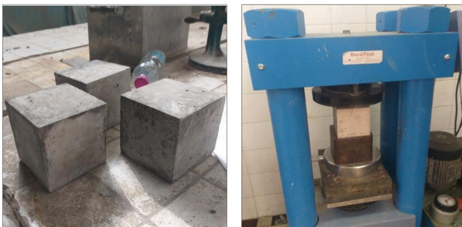
Figure V.7. Compression machine and specimens tested for crushing.
