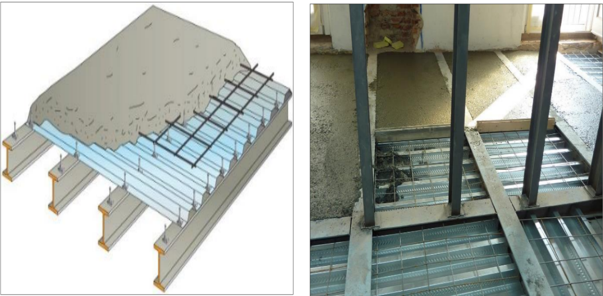
Figure I.9. Composite floors (steel-concrete).
