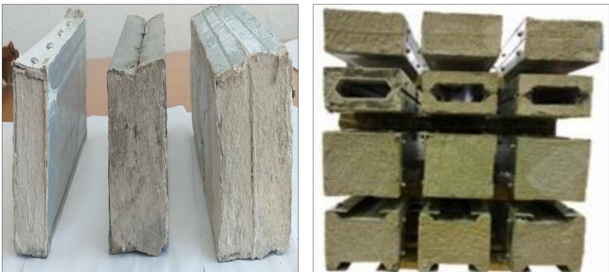
Figure II.12. Built-up cold-formed steel columns filled with concrete.
