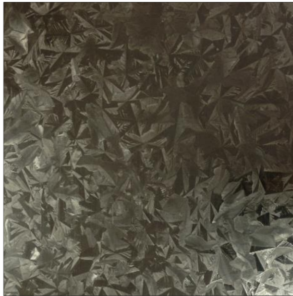
Figure I.13. Typical spangle of a galvanized coating.
