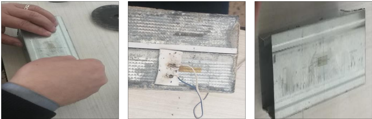
Figure V.8. The placement of the strain gauges.
