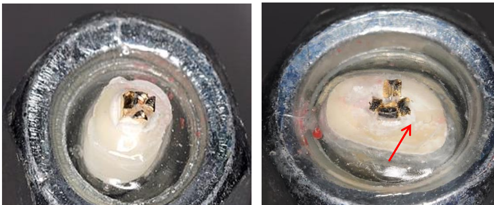
Figure 119. Tenons plaqués or (Gold plated) sous compression axio-apicale.
