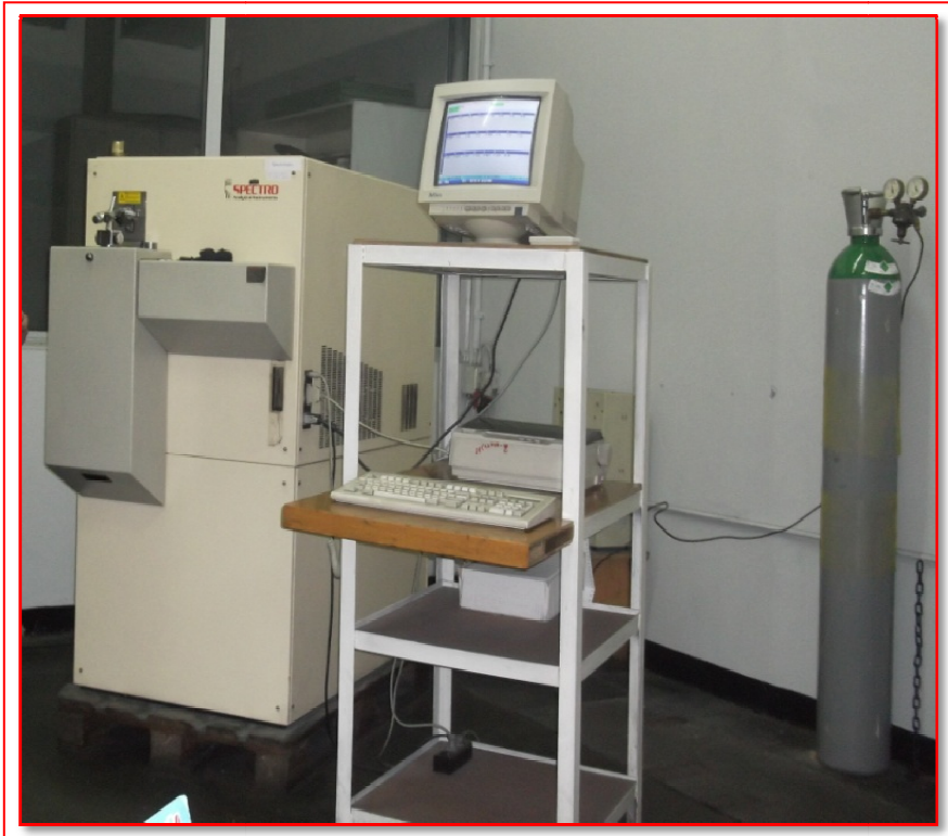
Figure II.9. Spectrométrie (SPECTRO Analytical instrument).
