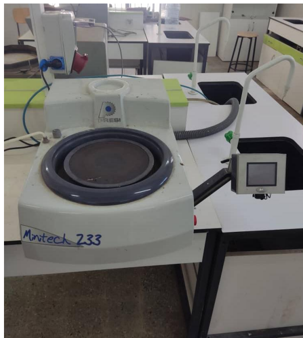
Figure II.12 : Machine de polissage minitech 233
