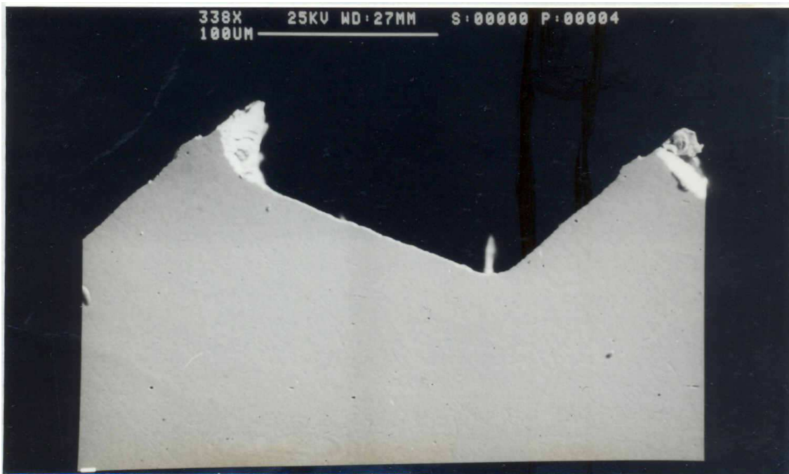
Fig. 52: Cross section of Annealed finish at a speed of 200m/min. Showing new shape of the feed marks.
