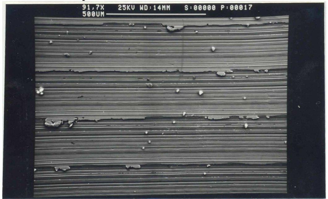
Fig 46: Surface finish of Annealed at a speed of 200m/min. Top of the feed marks.
