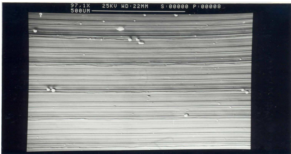
Fig. 41: Surface finish at cold drawn at a speed of 200 m/min. Using ground tool. r=1.27 \text{ mm}
