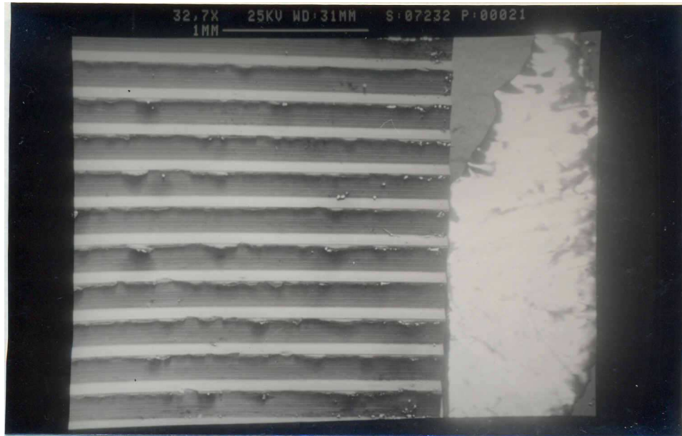
Fig. 59: Surface finish of cold drawn, machined at 350m/min. showing feed marks parallelisms.
