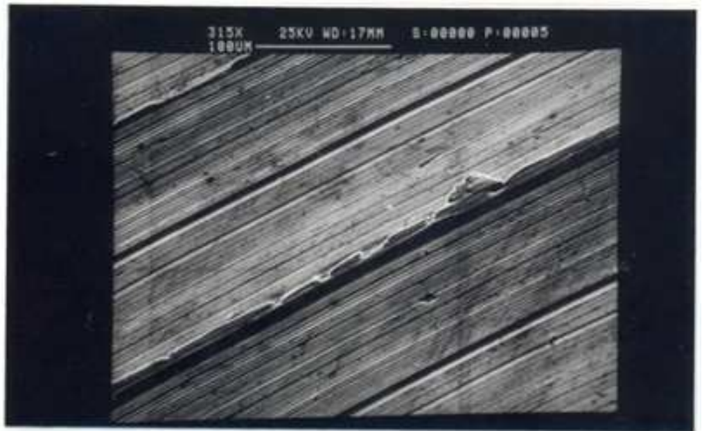
Fig. 34: Surface finish of Annealed at speed of 200 m/min. Dry condition.
