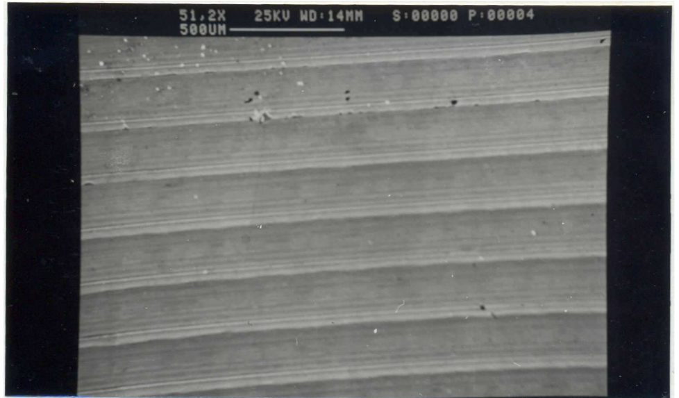
Fig. 26: Surface finish of 247165 cold drawn at a speed of 150m/min. Dry condition.
