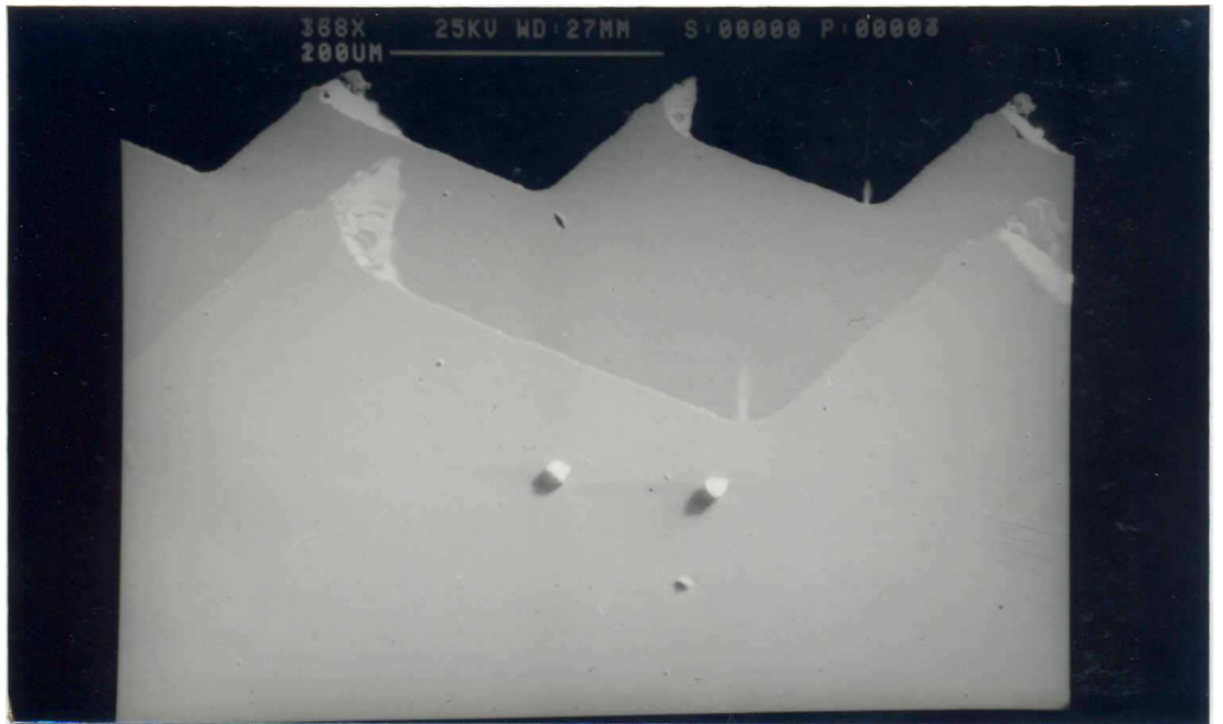
Fig 44: Surface finish of cold drawn at a speed of 200m/min. Cross section, showing real profile of the surface.
