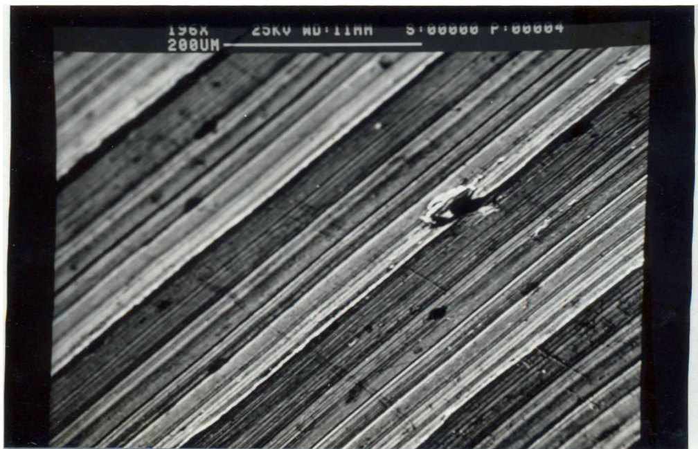
Fig. 33: Surface finish of Annealed at a speed of 150m/mn. Dry condition.
