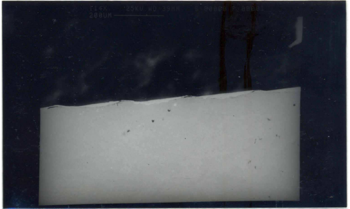
Fig 44: Surface finish of cold drawn at a speed of 200m/min. Cross section, showing real profile of the surface.
