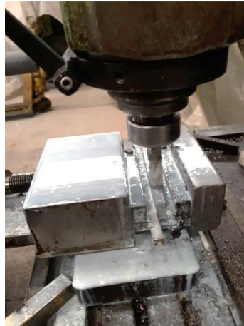
Fig.2.8: Surfacement des bords
