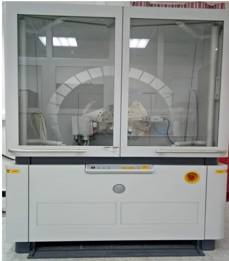
Figure II.3 : Diffractogramme type "PANalytical Empyrean" (LM2S- Annaba, Algérie).
