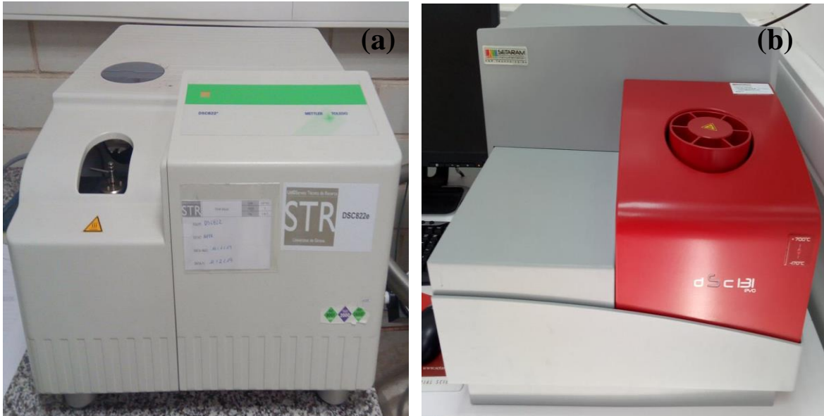
Figure II.10 : DSC822 de Mettler Toledo (Gironna, Espagne) (a), DSC131EVO (LM2S, Annaba–Algérie) (b).
